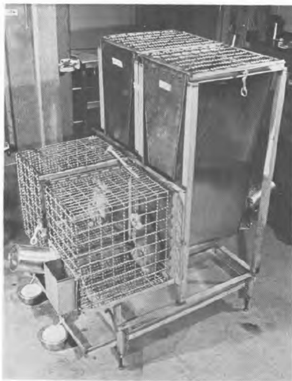
Figure 15-2. Vertical chamber apparatus with an attached living cage.
